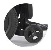
▼ As the drive wheel impacts the obstacle, some of the impact is absorbed by the compression of the front shock absorbers.
