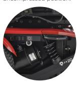
▼ Finally, the rear casters come into contact with the curb and the rear springs will absorb the impact and compress.
