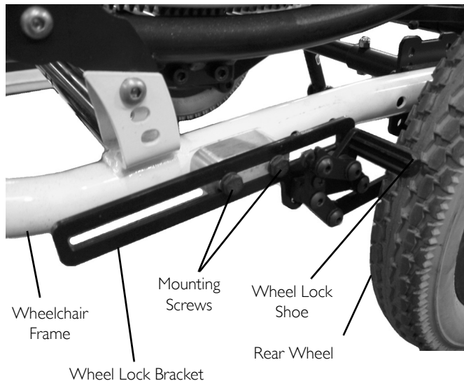
FIGURE 2 Wheel Lock Adjustment - Footlock
