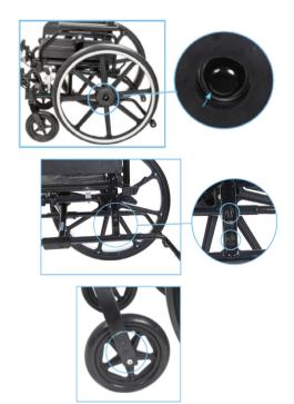
The 3 position front caster can be adjusted for positioning with the rear wheel. To adjust the front caster, loosen the bolt (outside of the caster) with an allen wrench (included). Remove the bolt and axle and place into the desired position. After the axle is placed in the new position, turn the allen screw clockwise to tighten.
