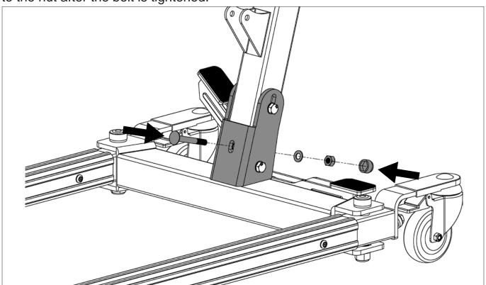
Step 5: Install the round plastic cover and plastic washers to the boom.
