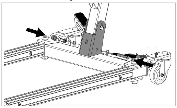
**Step 4**: Reinsert and tighten the carriage bolt to the front slot hole of the bracket, and the mast should be firmly secured to the base. Insert the black plastic cover to the nut after the bolt is tightened.
