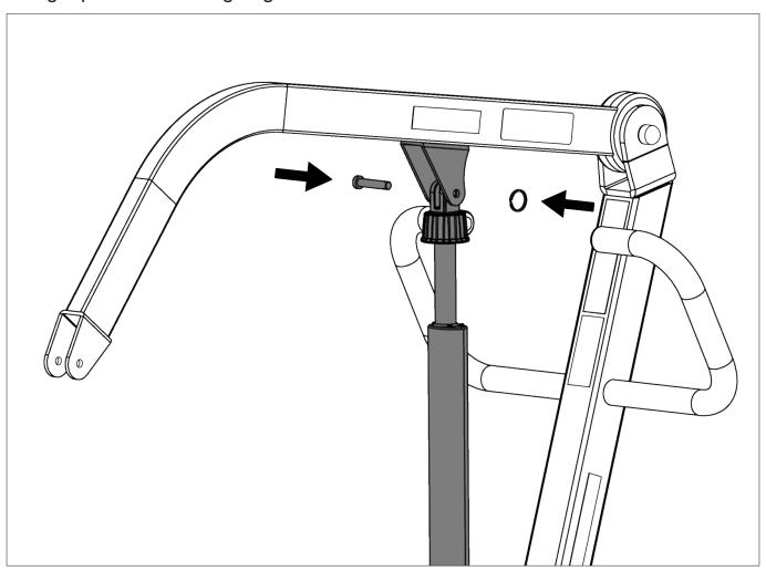
**Step 9**: Secure the spreader bar to the boom using a pin and retaining ring as follows.
