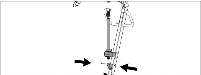
**Step 8**: Secure the upper end of the actuator to the bracket on the boom using a pin and retaining ring as follows.
