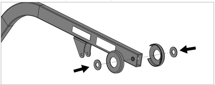
**Step 6**: Install the boom to the mast and align the holes. Then secure it by reinstalling the bolt, washer and nut. Once the screw is tightened using the EZ Tools, reinsert the plastic cap.
