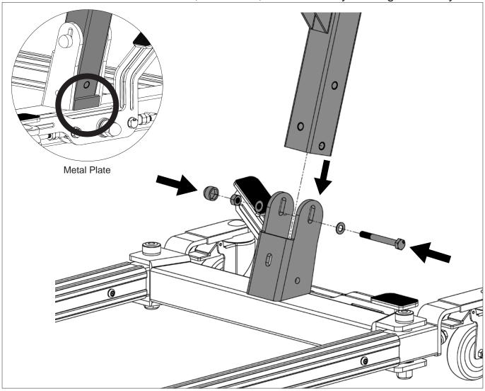
**Step 3**: Insert and tighten the other long hex head bolt, nut, and washers to the bottom hole on the side of the bracket to secure the mast. Insert the black plastic cover to the nut after the bolt is tightened.
