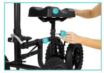
Take the brake line and secure it inside the two fabric straps you will find on the top bar of the frame as well as the steering column.
