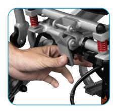
4. Plug in the joystick wire that is hanging down from the back of the chair into the port on the battery. Twist the locking collar on the plug to lock the plug into place.
