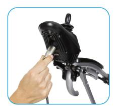
3. Insert the power plug from the Battery Charger into a standard 110v AC wall outlet. The Charge Indicator on the charger will illuminate blue to show that the battery is charging. It will take approximately eight (8) to twelve (12) hours for a full charge, at which point, the Charge Indicator will turn green.
