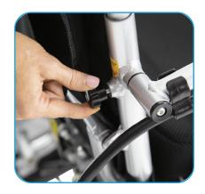
8. Switch the drive levers located behind each rear wheel from manual mode to drive mode. Drive Mode will allow you to Drive the scooter with the joystick. Manual mode will allow you to push the scooter manually as the brakes will be disengaged. Note that the scooter will not drive via the joystick while in Manual mode.
