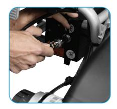
5. Slide the controller arm into the controller holder slot and then tighten down the arm using the twist lock screw.
